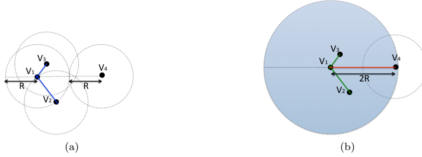
Fig. 1. (a) Scenario with three nodes ( v_1 , v_2 e v_3 ) within radio reach of each other and one distant node ( v_4 ). (b) Node v_1 uses nodes v_2 and v_3 as helper nodes to increase radio range thus reaching node v_4 .
