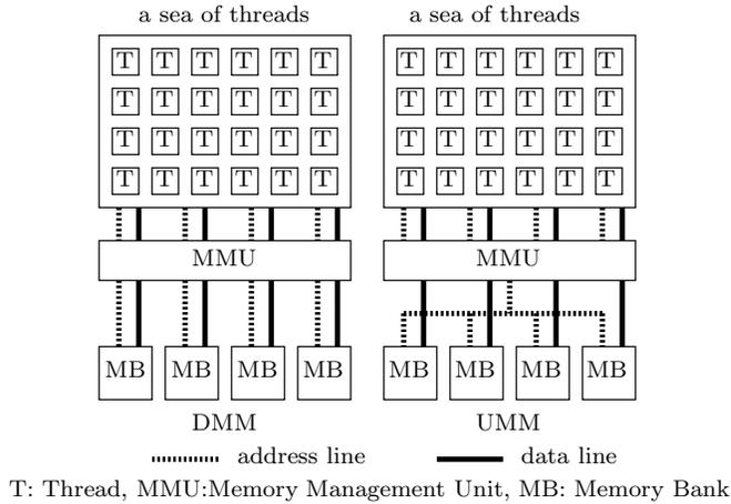
Figure 1. The architectures of the DMM and the UMM
