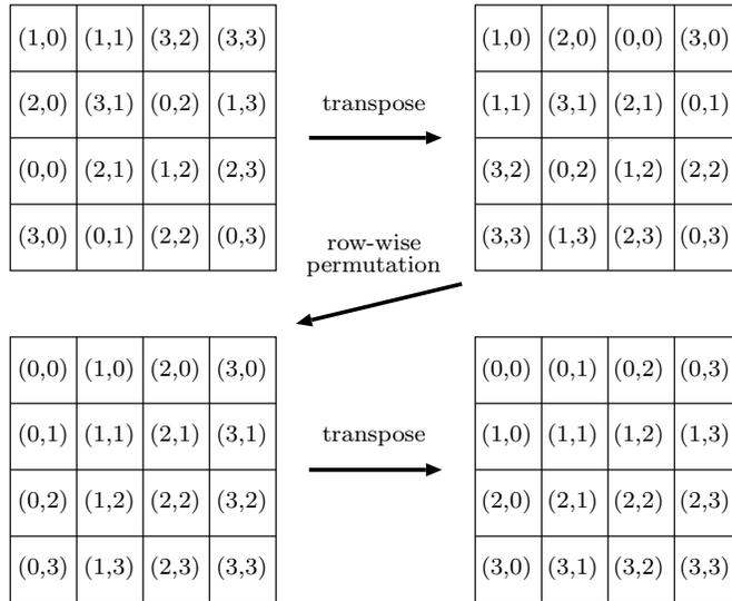
Figure 10. Column-wise permutation
