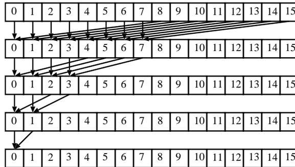
Fig. 4 Illustrating the summing algorithm for  $n$  numbers
