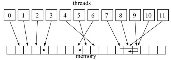
Fig. 3. An example of sequential memory access
