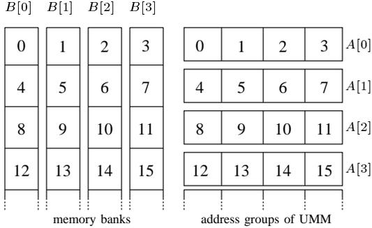
Fig. 2. The memory banks and the address group of the DMM and the UMM for  $w = 4$  banks
