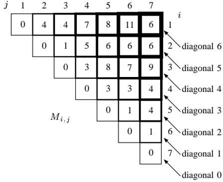
Fig. 8. The computation of  $M_{i,i+r}$  and the resulting values of  $M_{i,j}$
