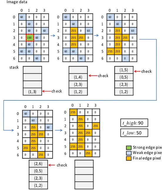
Fig. 5. Process of Hysteresis Thresholding
